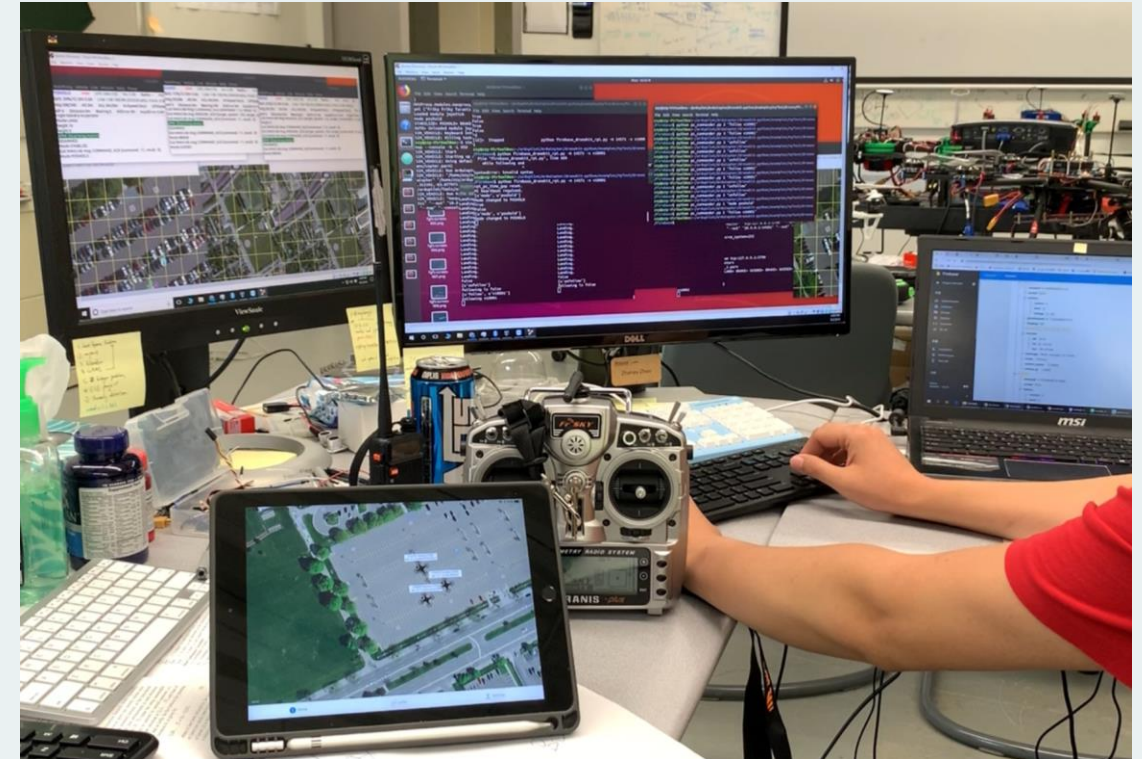
Simulated drones running with ArduPilot SITL (Software in the Loop)
